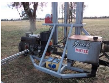
40' Auger 9" Fast Flow – Kohler motor.
