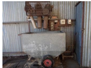
12T/hr Hammermill 50HP Motor
