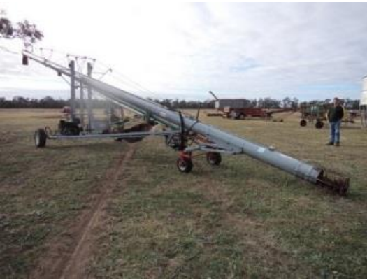
FINCH 60' Hydraulic ground drive 11" Auger – Lombardini motor.
